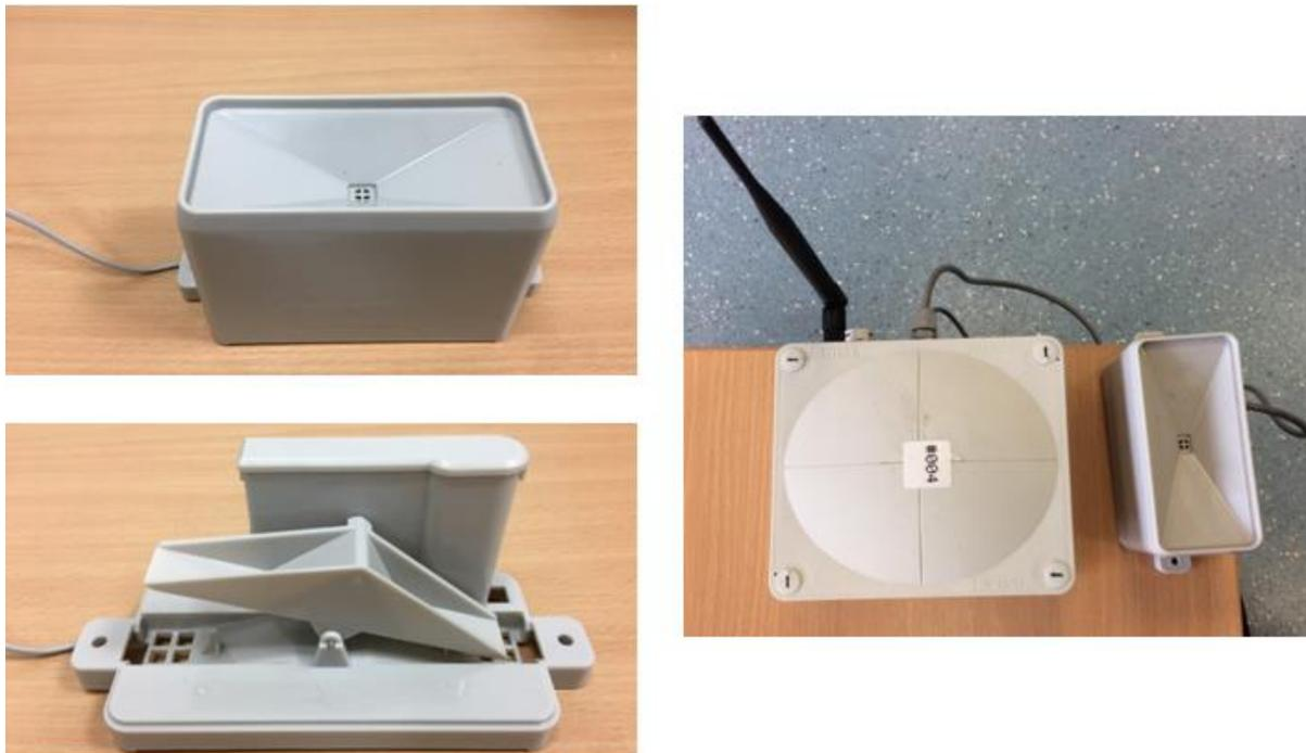
*Figure 1: Low-Cost Tipping Bucket Rain-Gauge (TBR) Complete with Transceiver (Right)*
